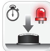
To save and return to the OPTIONS: Press and hold programming button until LED 1 turns solid RED.
