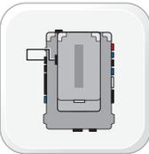
If the module has (1) red connector, connect the jumper cable as shown in the NOTE of the WIRING DIAGRAM. If the module has (2) red connectors, do not connect the jumper cable.
