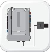
Connect the module to the computer with the WEBLINK cable. Flash the module with the latest firmware then flash the expansion pack.
