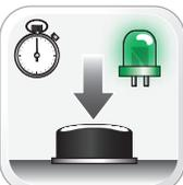
TO ACCESS THE MENUS: Press and hold programming button until LED 1 turns solid GREEN.
