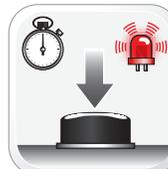
MANDATORY: EXIT MODULE NAVIGATION. Press and hold programming button for 7 seconds. LED 1 will flash RED rapidly. Release programming button. LED 1 will turn OFF.
