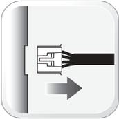
03 PRESS AND HOLD the module's programming button while connecting the BLACK 20-PIN connector.
