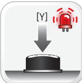
IN THE OPTIONS: Press the programming button as many times as the option number indicates. LED 1 will flash RED an equal amount of times continuously.
