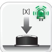
IN THE MENUS: Press the programming button as many times as the menu number indicates. LED 1 will flash GREEN an equal amount of times continuously.
