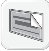
Put sticker 1 on a clean and visible surface in the engine bay and put sticker 2 under the dashboard near the OBDII connector.
